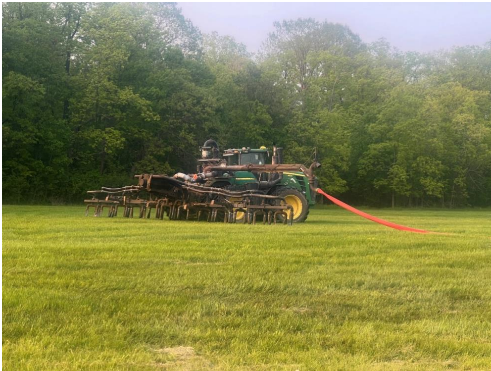
A dribble bar is the latest piece of manure equipment that allows the farm to quickly and efficiently apply manure close to the soil surface and on growing crops in-season.
